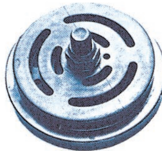
Valve after 1500 hours using CS300 oil
